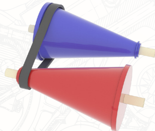
Friction cone variator with belt
