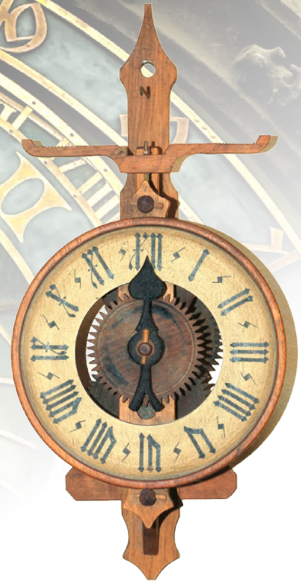
Old clock with an anchor escapement mechanism
