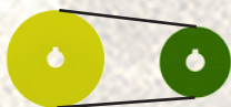
The belt on the second driven pulley. Position 2: the car goes faster
