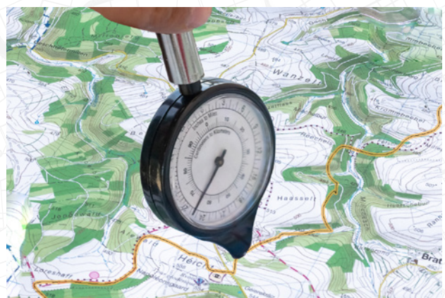
Pic 4. Measuring lines with a curvimeter
